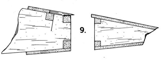
9.) Remove the rib fragments from the wing and flap, just as in book picture 44. for the ailerons.
