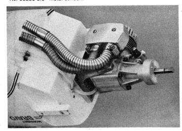
When making an initial installation of the S.T. 3000 or similar engine (when the 1/2" aluminum back plate would not be needed), select a long enough mount so that the firewall can be placed back away from the head. Cooling air flow will be better if the engine head is not right up
