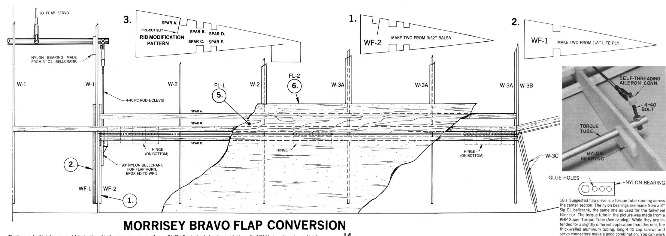
The flaps are built into the wing and detached from it in the same manner as are the ailerons. Study the aileron instructions and pictures in the book. They will help you understand the flap installation and the appropriate times to put in the extra flap
