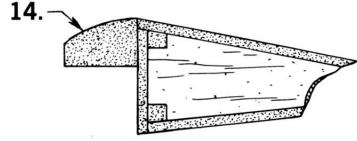
14.) Rough shape the block for clearance during movement.
