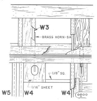
(e.) Use the aileron connecting rod pattern to make up the linkage to hook the top to the lower.
