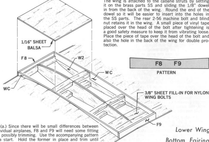
individual airplanes, F8 and F9 will need some fitting and possibly trimming. Use the accompanying pattern as a start. Hold the former in place and trim until there is a 1/16" space left for the bottom planking
