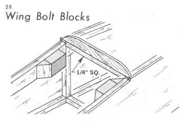
Epoxy Glue. (Not Kwik-Set, as more time than 5 minutes will probably be needed). Replace the wing and bolt it in position with the nylon wing bolts. This will force the FZ plywood saddles up tightly against the fuselage. If FZ does not seat down against the wing surface in some spots, drive a sliver of wood between the saddle and the fuselage to force FZ against the wing while the epoxy is setting up.
