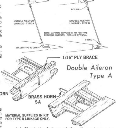
(a.) Sheet the bottom of the aileron horn compartment with 1/16" balsa.
