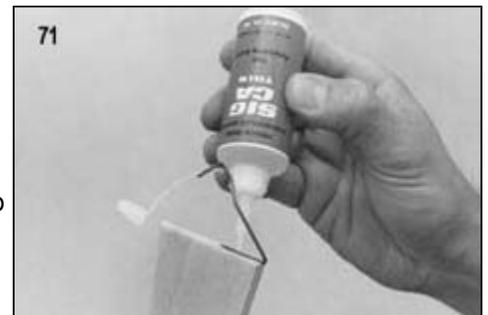
NOTE: Epoxy may be used in this step, but CA is faster and penetrates the entire tailwheel area, making it rock hard.
