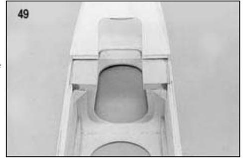
50. a. Fit the wing in place on the fuselage and check its alignment (see the General Alignment Drawing on page 20 of "The Basics of Radio Control" booklet). When you are satisfied that it is aligned correctly, tape it so that it can't move.
