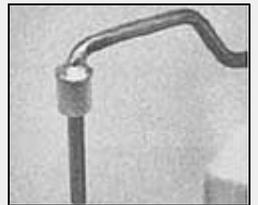
(2). Solder the washer, allow to cool, then remove the cardboard spacer. Grind off the excess wire and file the end smooth.
