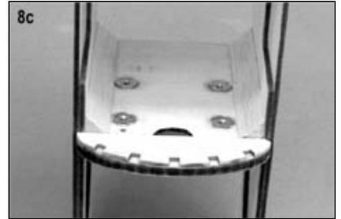
d. Now is a good time to install the tank floor. The height of the floor can be adjusted for different engines, just be sure to leave enough room for the tank. Block the tank in position with pieces of balsa, foam rubber or Styrofoam. If you use an oversize tank it may not be possible to install the tank later on, so hook everything up correctly now. If you use the recommended tank size the tank can be installed after the airplane is covered or painted.
