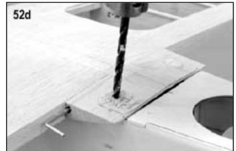
d. Seat the wing in the fuselage opening and tape securely in place - check the matchup of the alignment marks. With a #7 or 13/64" drill bit, drill two holes through the bottom wing and B-2. Make every effort to keep the holes perpendicular to the bottom of the wing so that the heads of the wing bolts will seat flat on the bottom of the wing.
