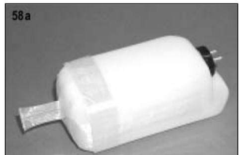
Access to the tank is easy if you use filament strapping tape to create a rear tab that allows you to grasp it and pull the tank out if needed. To do this, use alcohol to first clean the outside of the tank. Then wrap the length of the tank one or two times with strapping tape. Then wrap a third time, folding a 1-1/2" - 2" tab at the rear. The tab gives you a nice grip on the tank in order to easily pull it out.
