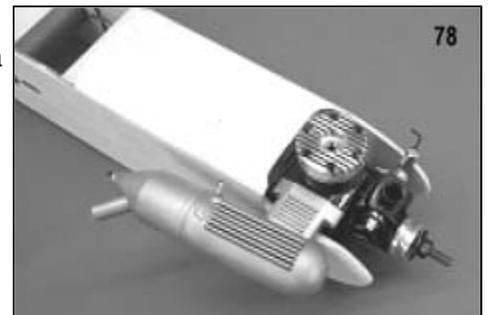
Some of the later two-stroke engines, with rear mounted remote needle valves, may require a hole in the left fuselage side for clearance. If your engine has this configuration, measure and drill the required hole. When these two issues have been taken care of, lightly sand these areas for covering.
