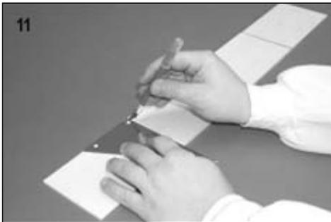
**BUILDERS TIP:** When edge gluing two pieces of sheeting off the structure, it is always best to sand the resulting joint smooth on both sides with a sanding block before gluing the sheet in place. This practice minimizes high and low spots, bumps, etc.
