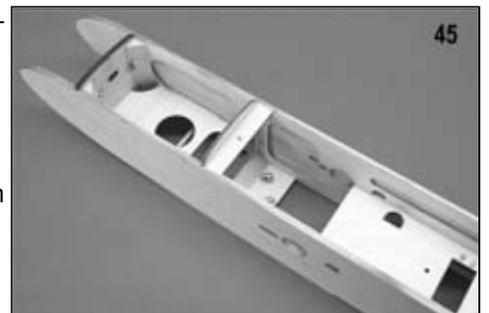
46. Glue the 1/8" ply tank floor in place to the fuselage sides, the back face of F-1 and the front face of F-2. Using the 1/8"x1/4"x36" balsa stock in your kit, cut a 3" length. This piece is now glued into the slots in the doublers, on the bottom of the fuselage, beneath the tank tray.
