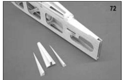
73. With the exception of mounting the stabilizer, fin and fairing blocks, the basic fuselage is complete and ready for final sanding. Use light weight filler to patch any holes, dings, etc. Use your sanding block and sandpaper to now sand the fuselage smooth. As shown on the plans, we sanded our fuselage with rounded edges on the bottom and at the nose. Take your time and do a good job.
