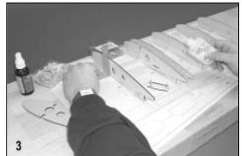
4. Glue ply rib W-2 in place, again using a triangle to ensure that it is exactly upright at 90 deg. and exactly over the plan. Ply rib W-1A is now glued in place over the spar.
