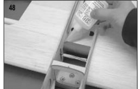
Repeat the procedure to mount the remaining wing panel. Hook a #64 rubber band to one of the J-hooks and stretch the rubber band three times between each hook to seat the wing panels in place. Check the relationship of the wing panel root ribs to the fuselage sides - they should be flush with no gaps. With the wings still attached, apply glue to the inside female wing tube/fuselage side joints. Also apply glue to the female wing tube, where it meets the front edge of the servo tray.
