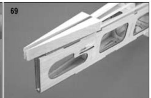
70. Use a razor plane or hobby knife to roughly carve the fairing blocks to match the lines of the fuselage. Use 80 grit sandpaper to further shape the fairing blocks to the cross section shape shown on the plans. When the shape is close, use 220 grit sandpaper to sand the rear stringer area and the fairing blocks smoothly together. Done properly, the whole thing looks almost one-piece.
