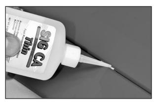
e) Turn the part over and glue the other side of the hinge. Continue this process until you have glued both sides of all the hinges! Keep a rag handy to wipe off any excess Thin CA glue. (If you get some glue smears on the plastic covering, don't worry about them right now. Once all the hinging is done, you can clean the smears off the covering with CA Debonder).
