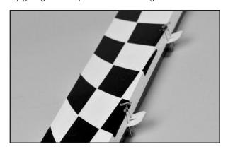
d) Flex the aileron down and hold it in this position. Remove the pins from one hinge and then carefully apply 3-4 drops of Thin CA glue directly onto the hinge in the gap. You will notice that the glue is quickly wicked into the slot as it penetrates both the wood and the hinge. We suggest using a fine tipped applicator on the glue bottle to better control the flow of glue.
