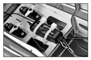
**NOTE:** If you are not using BEC, but are instead using a separate receiver battery, you can mount your on/off switch in the pre-cut hole in the fuselage side. You will need to open up the covering where the hole is cut in the wood.
