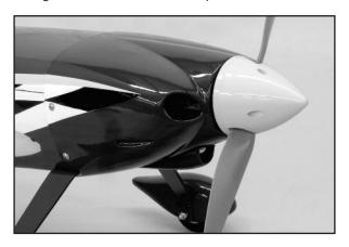
□ 33) Mount a suitable propeller on your motor with the included spinner. Be sure to balance the prop before installation.
