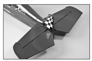
□ 17) Hinge the rudder to the fin and the rear of the fuse-lageusing the same techniques you did for the other hinges refer to page 5 of this manual. Make sure to line up the top of the rudder flush with the top of the fin. This will ensure the tail-wheel bracket lines up correctly. Let the hinges dry adequately before proceeding.
