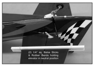
c) Inside the fuselage, hold the pushrod wire over the elevator servo output arm and mark the wire where it crosses over the outer hole in the servo arm.
