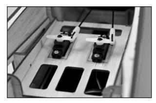
□ 23) Locate the pre-cut pushrod exit hole for the rudder on the left side of the fuselage at the back of the plane and repeat step (22) in its entirety to install the rudder pushrod.
