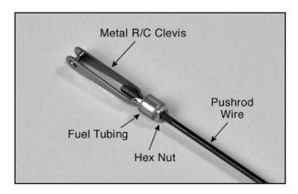
b) Clip the metal clevis into the last hole in the nylon control horn. Lay the other end of the pushrod wire over the outer hole in the servo arm. Use a felt tip pen to mark the wire where it crosses the hole. Use a pair of pliers to put a sharp 90-degree bend in the wire at the mark.
