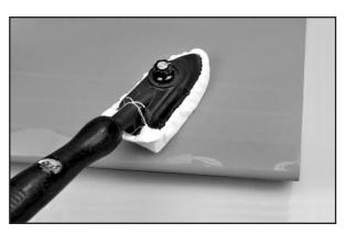
After you have all the covering secured onto the solid areas, turn the temperature of the iron up to approximately 300°F - 320°F (149°C - 160°C). This is the correct temperature for shrinking the covering material.
