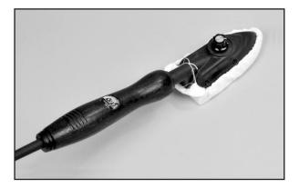
We suggest using a model airplane covering iron for this process. Cover the iron's shoe with a thin cotton cloth, such as an old t-shirt, to prevent scratching the covering as you work. After covering your iron, the next step is to set the iron to the correct temperature. This is critical for achieving a good result! The iron should be set to about 220°F - 250°F (104°C - 121°C) as measured on the bottom of the iron using a thermometer.
