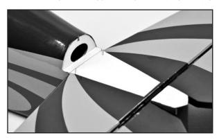
for this job to allow time to position the stab accurately and make any final adjustments that might be needed. Apply the glue to both sides and reset the stab in place. Use pins to hold it in place. Recheck the alignment. Wipe away any excess epoxy with rubbing alcohol and a soft paper towel. Allow the glue to set completely.
