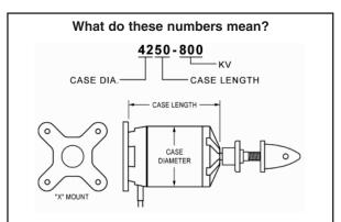
**Note:** This numbering system is very common, however there are exceptions. For instance, some motor manufacturers will list the actual diameter of the stator (armature) inside the motor instead of the case diameter. Some may list the length of the stator inside the motor instead of the case length. Some will give you both if you dig far enough into their specs. Make sure you understand the motor manufacturer's numbering system when shopping for a motor.
