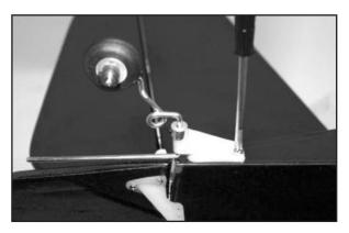
c) Slide the bearing onto the wire that runs along the bottom of the rudder. The tab of the bearing will be epoxied into the slot that is precut on the bottom of the rudder. Test fit the assembly to make sure everything will line up.
