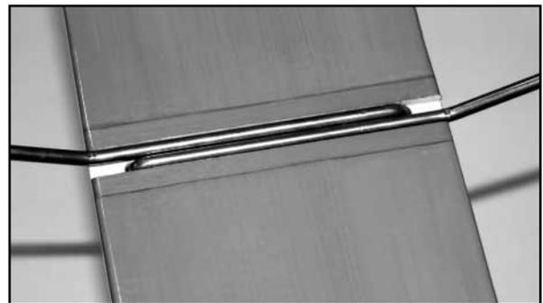
4) Place the two nylon landing gear retaining straps over the main gear wires as shown in the picture. Mark, then drill four 1/16" dia. pilot holes for the screws. Use four M2.5 x 16mm PWA Screws to mount the straps.
