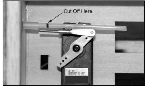
7) a) Remove the R/C link from the throttle arm, and then pull the throttle pushrod tube out of the sleeve. Use a razor blade to cut the pushrod tube at the mark made in the previous step.
