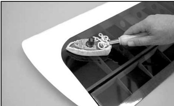
If wrinkles keep coming back on the tail surfaces, you may need to "ventilate" the areas between the ribs. Otherwise the air that is sealed in those relatively small areas will expand when the heat is applied and actually cause the covering to stretch instead of shrink. Use a pin to poke a tiny hole in the covering between each rib, on the bottom of the part. That will let the expanding air escape and the covering to shrink properly.
