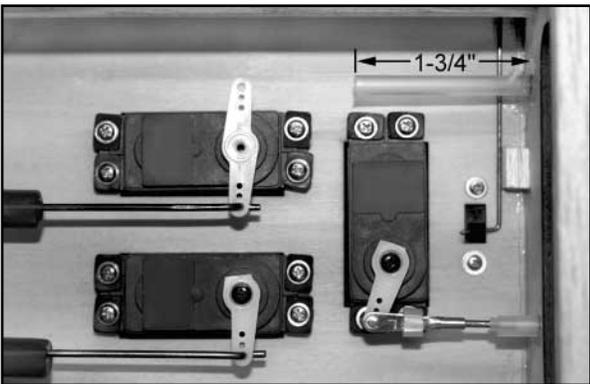
5) a) From the front of the airplane, insert the plain end of the nose gear pushrod inside the outer sleeve and slide it all the way back.
