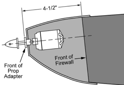
1) There are four sets of "cross-hairs" etched on the front of the plywood firewall to mark the locations of the mounting holes for the Maxx Products #ACC3958 Motor Mount. To install this mount on the firewall you will need to purchase (4) 4-40 x 1/2" Socket-Head Bolts, (4) #4 Flat Metal Washers, and (4) 4-40 Blind Nuts. Drill the four mounting holes with a 9/64" or #27 drill bit.
