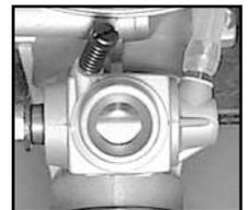
Use the EPA (End Point Adjustment) feature of your transmitter to accurately dial-in the desired servo travel. Also make sure there is no binding in the throttle linkage, which could cause unnecessary battery drain. Understand that the final throttle set-up will be done after the engine is broken-in and running.
