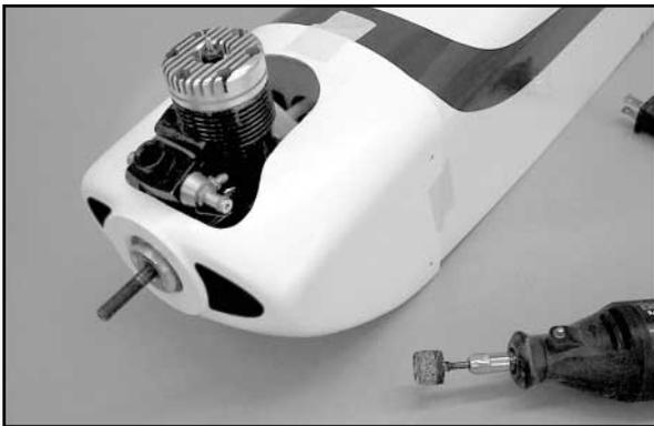
3) When satisfied with the opening in the cowling, mount the cowl to the fuselage with the four M2.6 x 10mm PWA Screws provided.
