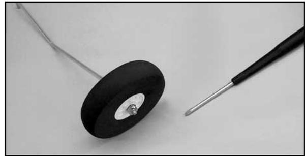
3) Turn the fuselage upside down on a padded work surface for installing the main landing gear. If your receiver antenna is over the landing gear slot, remove the rubber band holding it in place and move it out of the way temporarily. Fit the two main landing gear wires into the holes and slot in the bottom of the fuselage.
