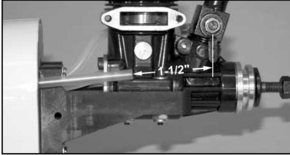
4) Screw an M2 x 7/8" threaded stud into one end of the 1/8" od x 19-3/4" nylon pushrod tube - thread it in at least 1/4" or more. Then screw a metal R/C link halfway onto the stud. NOTE: If the threaded stud screws into the plastic tube too easily, not getting a good "bite" in the plastic, put a little epoxy glue or medium CA on the threads and in the end of the tube before screwing it in.
