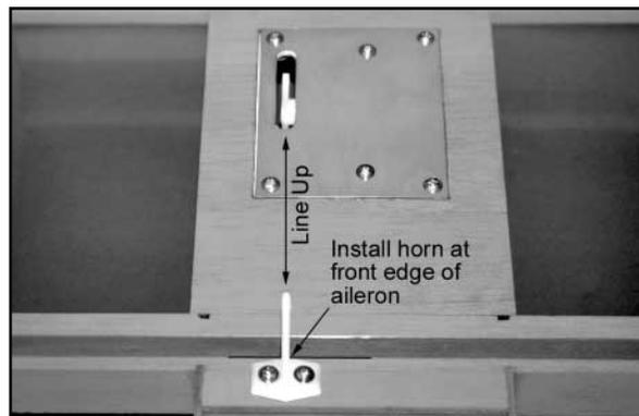
7) Before installing the pushrods you should hook your two aileron servos up to your radio system to check their operation.
