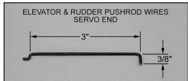
e) Mix a small amount of 5-minute epoxy. Apply the glue in the channel and in the hole in the pushrod. Also apply epoxy to the 90° bent end of the wire pushrod. Insert this end into the hole and channel, pressing it firmly in place. Wipe off any excess glue and allow the glue to set.
