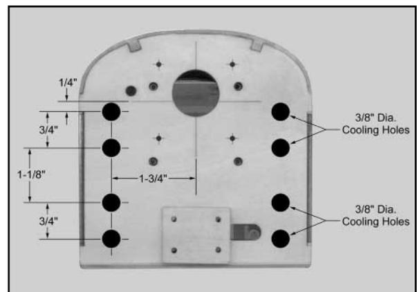
4) Bolt your motor and mount to the firewall. Use thread lock compound (not supplied) on all the bolt threads.
