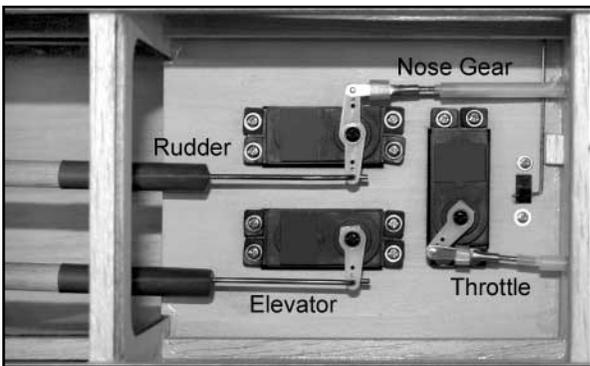
10) Turn on your radio and test the action of the steerable nose gear. It should be smooth and free of any binding. You can refer ahead in this manual to the section on "Control Surface Travel" and adjust the rudder and nose wheel travel now.
