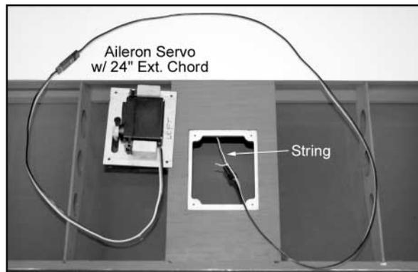
b) Break loose the balsa stick that has the opposite end of the string tied to it - from its location at the inboard end of the wing panel. Begin carefully pulling the string and the aileron chord through the wing towards the end of the wing panel. You may occasionally feel like the wire has become stuck inside the wing.
