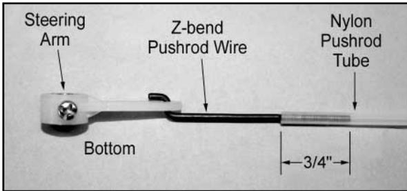
4) The outer sleeve for the nose gear pushrod is already installed in the fuselage, but not glued. Position the sleeve so the front end sticks out in front of the firewall about 1/8". Mark and cut off the servo end about 1-3/4" aft of the fuselage former in front of the servos. Secure the sleeve by gluing it to the two formers that it passes through inside the fuselage.
