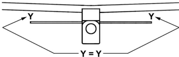
When satisfied with the alignment, remove the stabilizer from the fuselage in preparation for gluing on permanently.
