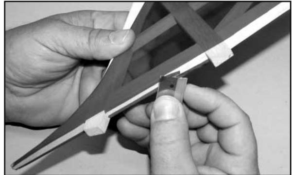
5) Apply epoxy glue to the bottom of the fin, including the tabs that fit into the slots in the stabilizer and fuselage. Press the fin/rudder assembly in place. Use masking tape to hold the fin in correct position. Double check the alignment of the fin - it should be perpendicular (90°) to the stabilizer. Adjust the tape as needed to hold it in position. Use alcohol and a paper towel to wipe off any excess glue. Allow the glue to dry completely before proceeding.
