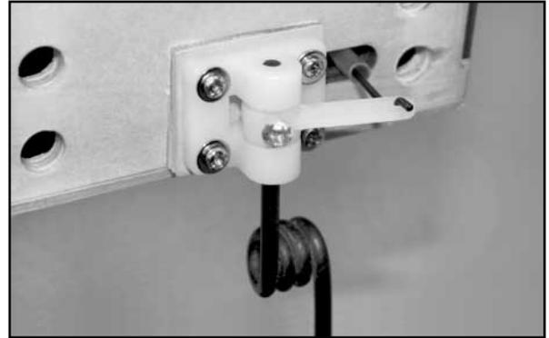
6) Align the nose wheel so it points straight ahead. Adjust the steering arm position on the nose gear wire so that the outer hole in the arm is about 7/8" away from the front of the firewall when the wheel is pointed straight ahead.
