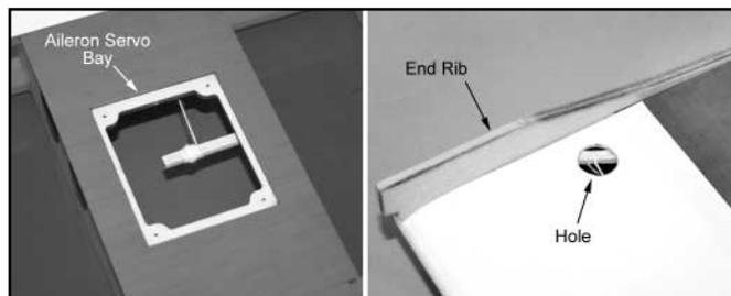
a) In the servo bay, gently break the small balsa stick loose from the wing structure. Pull it out and unwrap the extra string. Remove the wood from the string and discard it. Tie the end of the string securely to the end of the servo wire, as shown.
