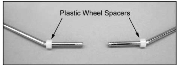
2) Install a 3-1/2" dia. wheel on the axle and slide it up against the plastic space. Then install a wheel collar and tighten the set screw. Make sure the wheel turns freely. Repeat the process to mount a wheel on the other main gear wire.
