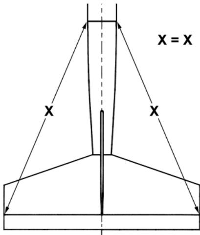
Also check the alignment of the stabilizer from the front view. Mount the wing to the fuselage, using the two 1/4-20 x 1-1/2" nylon wing bolts provided. Place the model on a flat surface and orient it to allow you to view the airplane from the front from a distance of 10 feet or so. With the stabilizer squarely in place and pinned, view the airplane from the front and rear. The stabilizer should be equally aligned with the wing - not tilting one way or the other. If it is tilting, correct it.
