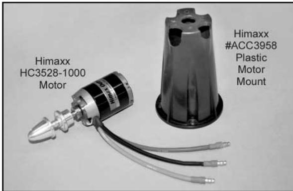
**IMPORTANT NOTE ON MOTOR MOUNTS:** If you are using a different brand electric motor or motor mount, you need to make sure that the combination you select can provide exactly 4-1/2" distance from the front of the prop adaptor to the front of the firewall (i.e. back of the mount). 4-1/2" is the distance needed for the cowling to fit properly.
