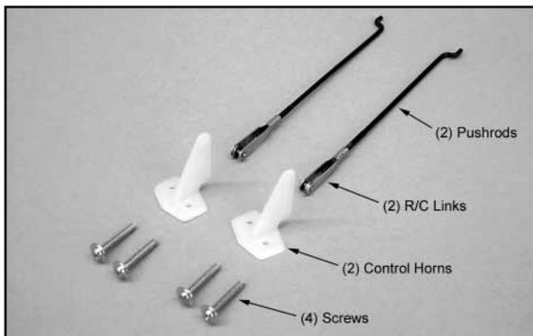
6) Install a Nylon Control Horn on the bottom of the aileron. Make sure the horn is directly in line with the servo arm, and that the base of the horn is right at the front edge of the aileron.
