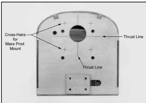
*NOTE: If you are using a different mount, line your mount up on the firewall according to the horizontal and vertical thrust lines that are etched in the plywood. Then drill appropriate holes where needed for your mounting bolts.*
