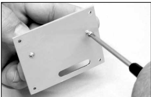
f) Mount your servo to the hatch, using the screws that were provided with the radio system. Be sure to drill pilot holes in the mounting blocks before screwing the servo in place.
