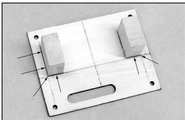
e) M2 x 8mm PWA Screws are provided to reinforce the mounting of the hardwood servo blocks to the hatch. Use a ruler to find the center of each block and mark it on the covered side of the hatch. Drill a 1/16" dia. pilot hole about 1/4" deep, through the hatch and into the mounting block. Install a screw in the hole. Repeat to install a screw in the other mounting block.
