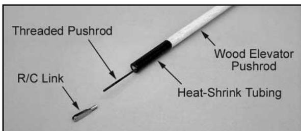
f) The elevator pushrod is ready to be installed in the airplane. Thread a metal R/C link onto the threaded pushrod wire, about
