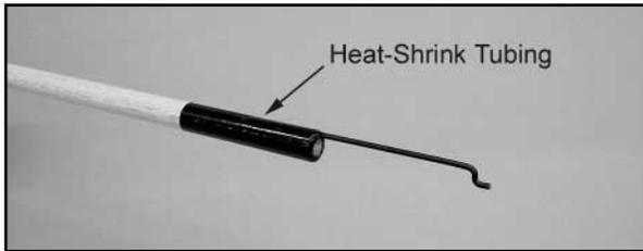
4) With the servo ends of both the elevator and rudder pushrods completed, the opposite ends are now assembled. This is where the two pushrods become different. In this step, we will complete the ELEVATOR PUSHROD and install it in the airplane.
