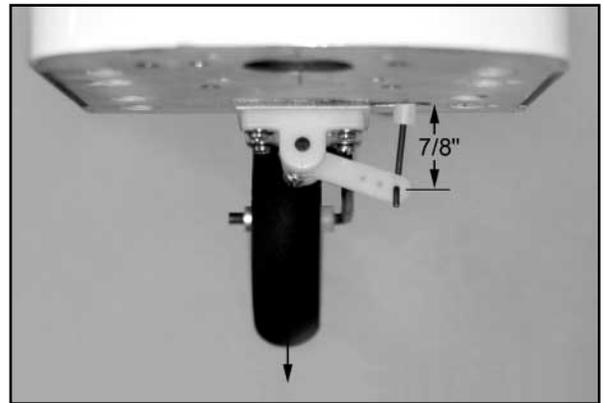
7) Use a marker pen to mark the location of the set screw on the nose gear wire. Remove the wire and file or grind a flat spot in the wire for the set screw to rest in. Then reassemble the parts, tightening the set screw securely. The flat spot will help insure that your nose gear steering doesn't slip.
