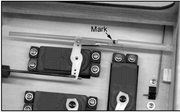
d) Take the R/C link and stud off the servo arm and screw the stud into the pushrod tube. NOTE: It's easier to do this if you remove the steering arm so you can take the pushrod out of the sleeve. That makes it easier to screw the threaded stud (alone, without the R/C link attached) into the servo end of the pushrod tube. When done, put everything back together and re-attach the R/C link. Make sure everything is tight, and that you've got all the servo arm screws installed.
