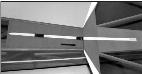
4) Use a very sharp blade (single-edge razor blade shown) to slice off any excess covering material on the bottom of the fin, in order to maximize the gluing area where it mates to the stab and fuselage.
