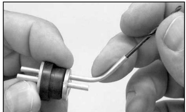
6) Test fit the completed stopper assembly into the neck of the fuel tank. Rotate the stopper so the aluminum tubes are horizontal at the bottom of the stopper. Hold the tank up to a strong light and look inside to see if the vent tube is close to the top of the tank. If not, adjust the bend in the vent tube as needed.
