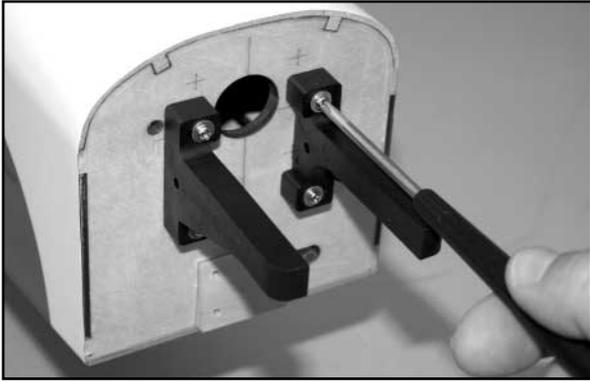
3) Slide the engine forward or aft on the engine mounts until the front of the engine's thrust washer is 4-1/2" from the front of the firewall.
