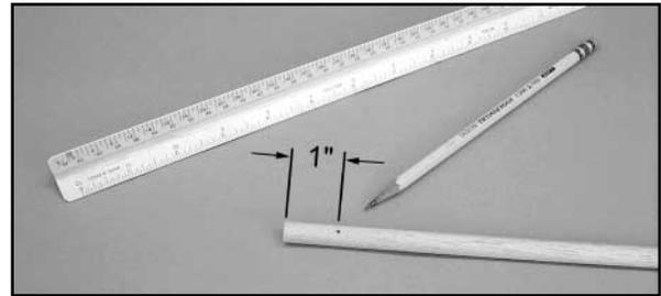
b) Use a 5/64" drill bit to drill a hole all the way through the pushrod at the mark just made.
