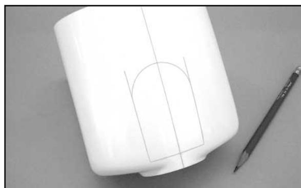
Then take width and length measurements off your engine and transfer them to the top of the cowl, using the centerline as the base reference point. The simple pattern shown in the previous photo was quickly made by measuring the diameter of the engine head and the overall length of the engine. It will serve as an undersize starting point for removal of material.
