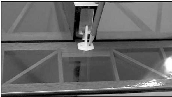
2) Mount a nylon control horn on the left side of the rudder with two M2 x 20mm bolts and a nylon control horn base, using the same techniques you did in the previous step for the elevator horn.
