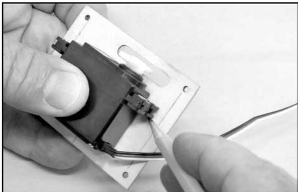
d) Use Medium CA or epoxy to glue two Hardwood Servo Mounting Blocks in position on the hatch, right up against the lines you drew on the hatch, as shown. Let dry.
