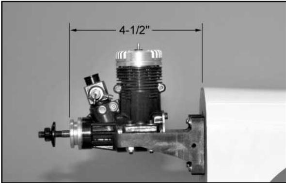
4) Double check to make sure that the engine is pointing exactly straight forward, and then mark the locations of the engine mounting holes onto the beams of the engine mounts, using a center punch or sharpened nail.
