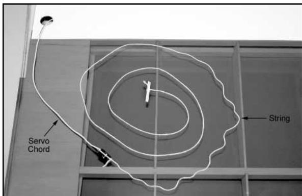
d) Repeat this step to pass the other aileron servo wire through the other wing panel.
