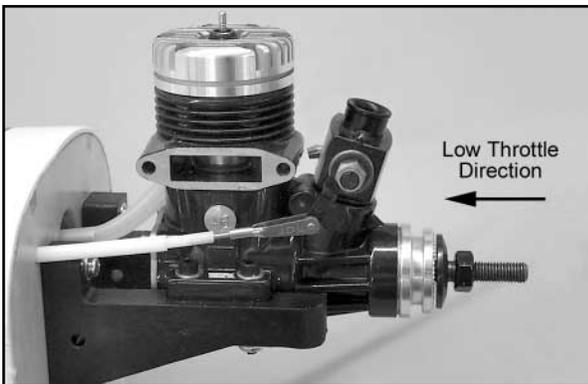
**NOTE:** Most 2-stroke R/C engine carburetors will provide low throttle when the throttle arm is pulled fully back toward the rear. Check your carburetor and confirm the correct direction of travel for "low" and "high" throttle movement and then check the throttle servo to be sure it also moves in the right direction.
