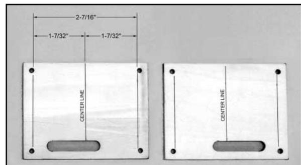
c) Hold one of the servos up against the back side of the hatch, with the servo arm centered in the pre-cut slot in the hatch. Mark the bottom of the servo grommets onto the hatch. Then draw a pencil line across the hatch at this mark (this line runs across the hatch, perpendicular to the other lines you drew).
