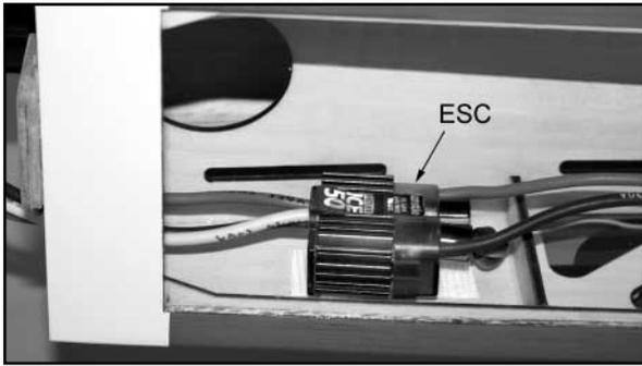
7) Pass the motor leads from the ESC through one of the cooling holes you made in Step 3. Connect the leads to your motor. Use the radio system to operate the motor and check the direction of rotation. If you need to reverse the rotation, refer to instructions that came with the motor and ESC.
