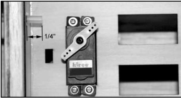
3) Cut off the front end of the sleeve approximately 1-1/2" away from the center of the throttle arm. Glue the sleeve to the firewall.
