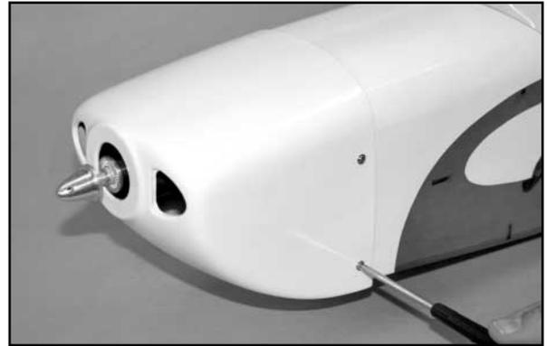
11) **OPTIONAL SPINNER:** A 2" dia. spinner is included in this kit. No doubt it will be used by almost everyone who is installing a glow engine. However with an electric motor you may prefer to not use the spinner in order to allow more cooling air to flow into the cowling. The opening between the prop shaft and the cowling (which a spinner would cover up) allows a significant amount of air to flow in directly onto the motor, to keep it running cool.
