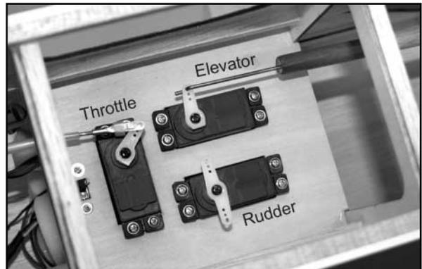
5) Next, we will complete the RUDDER PUSHROD and install it in the airplane.
