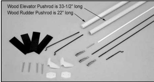
1) Mount a nylon control horn on the bottom of the elevator with two M2 x 20mm bolts and a nylon control horn base.
