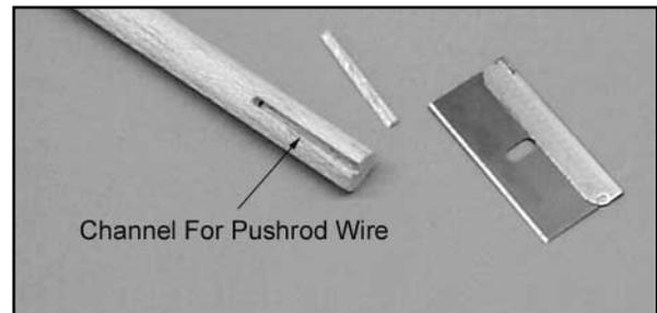
d) Prepare a 2mm x 4" long pushrod wire for mounting in the channel. Use a ruler to measure exactly 3" back from the z-bend. At this mark, use pliers to bend the wire downward 90°, inline with the z-bend. Use diagonal cutters to trim the bent end, leaving 3/8".
