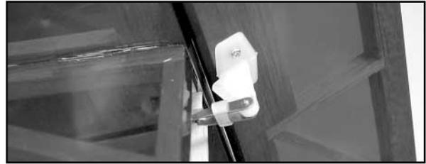
g) Turn on your radio system and make sure the elevator trim is centered. Then check to see that the elevator servo arm is also centered, at 90° to the servo. If not, reposition the servo arm.
