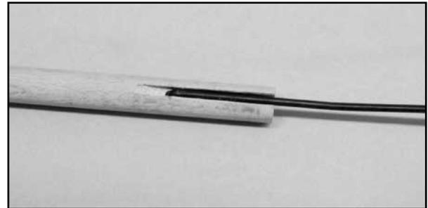
When the glue has cured, cut two 2" lengths of heat shrink tubing from the supplied material. Slip a piece of heat shrink tubing over the glued wire at one end of the wood pushrod and use a heat gun
