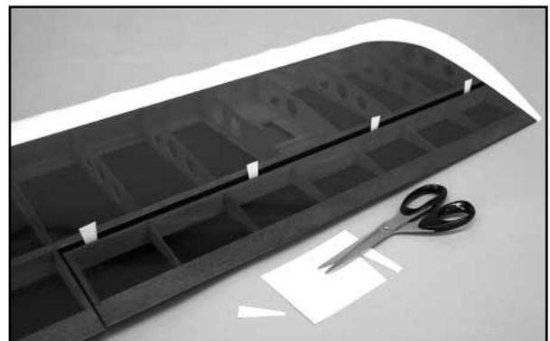
❑ 3) Flex the aileron downward, exposing the hinges between the wing and the aileron. Hold the aileron in this position with a
