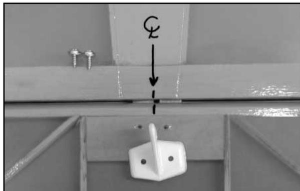
□ 5) To create the best wood-to-wood bond, the covering material on the bottom center section of the stabilizer needs to be removed. First, use a cloth-covered heat iron to firmly adhere the covering to the wood in the center section area. Place the stabilizer onto the fuselage at the rear and carefully center it. Use a non-permanent marker pen to trace the fuselage side locations
