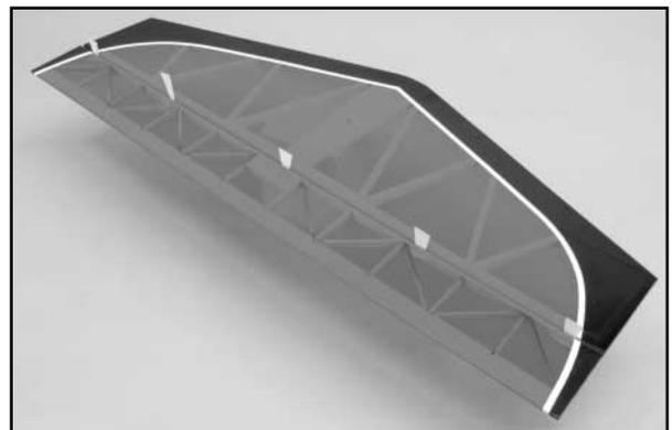
□ 3) Because it is much more convenient to attach the control horns to the rudder and elevators at this point, we suggest doing this now. As shown, the nylon rudder control horn is positioned on the left side of the rudder, at the bottom leading edge of the rudder.
