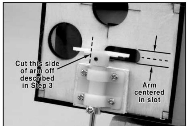
□ 3) With the nose gear assembly now in place, a simple precaution should be made to ensure that neither the steering arm or the wheel collar can slip out of position. We suggest using a Dremel® Tool or a small file to grind a small "flat" in the nose gear wire, directly at the setscrew locations.
