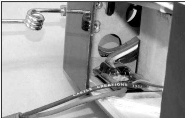
□ 4) The receiver is now mounted in the fuselage on top of the battery tray, again using a 1-1/2" length of the provided Velcro®
