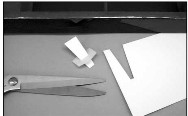
❑ 2) Press the three hinges into the slots in the wing panel up to the hinge slot cutout. Place a card wedge into each hinge and then, press the aileron in place onto each exposed hinge half, up to the card wedges. Slide the aileron left or right to center it within the wing panel aileron bay. The hinges are now in proper position for permanent mounting.
