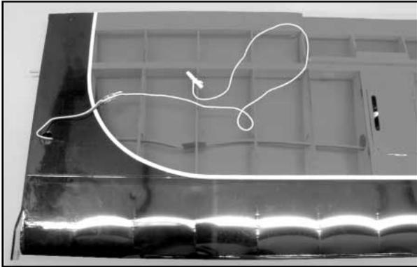
Repeat this process to route the servo extension lead and to seat the aileron servo mount/hatch in the opposite wing panel. Temporarily tape the loose aileron extension leads to their respective wing panels. The two aileron servo hatch/mounts can now be secured to each wing panel with the screws removed earlier.
