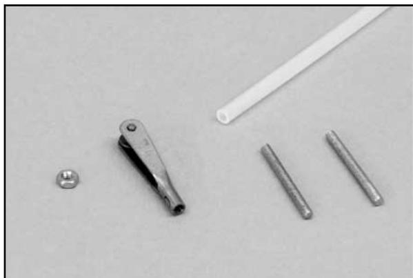
Thread one of the M2 x 24 mm studs into one end of the nylon pushrod tube to a depth of about 3/8". As shown, this is easy to do by using an electric drill. Chuck the stud firmly into the drill and then simply use the power of the drill to thread the stud in place into the nylon tube.
