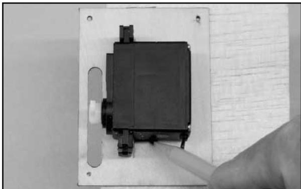
❑ 8) Use epoxy or thick CA to glue two 20 mm x 20 mm x 10 mm hardwood servo mounting blocks to each aileron cover as shown. When the glue has set, the servos can be mounted to the hatch/mounts using the servo mounting screws that came with your radio system. Use a 1/16" dia. bit to drill pilot holes for the servo mounting screws.
