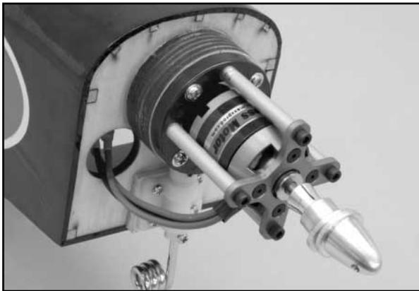
□ 6) The three motor wires from the ESC are now connected to the appropriate three wires from the motor, through the round laser-cut hole in the firewall.
