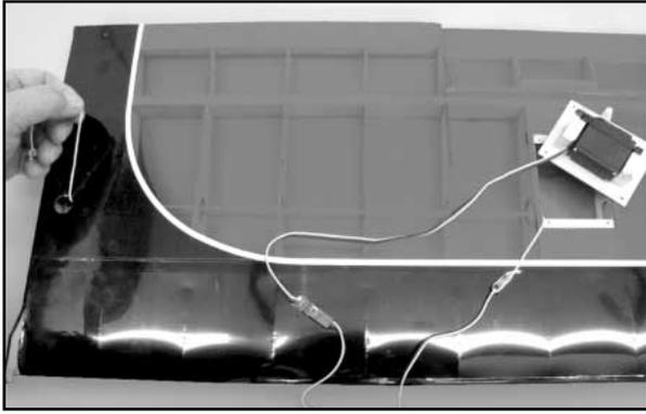
When the extension connector is pulled through and out of the hole, pull the rest of the lead assembly out of the hole while fitting the aileron hatch in place into the opening at the outer end of the panel.
