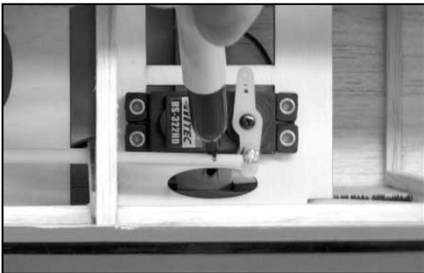
Remove the tape holding the nose wheel in place and disconnect the RC link at the steering arm and remove the nose gear pushrod tube. Cut the tube at the mark just made. Chuck the remaining M2 x 24 mm threaded stud into an electric drill and thread the stud into the servo end of the nylon pushrod tube to a depth of about 3/8". Reinstall the nylon pushrod tube through the firewall opening and back into the 5 mm pushrod housing tube. Reattach the RC
