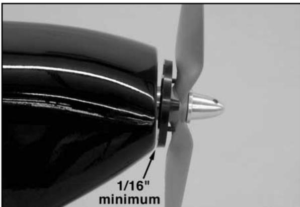
Use pieces of tape to firmly hold the cowl in this position. Use a 1/32" bit to drill four pilot holes through the pre-drilled holes in the cowl, into the fuselage. Use the four provided T2.6 x 8 mm PWA screws to now mount the cowl in place to the fuselage.
