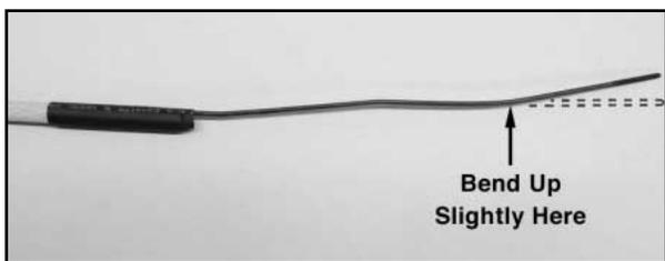
Insert the pushrod into the fuselage through the wing opening, guiding it back toward the tail. Maneuver the pushrod until the threaded pushrod end exits the slotted hole at the top rear of the
