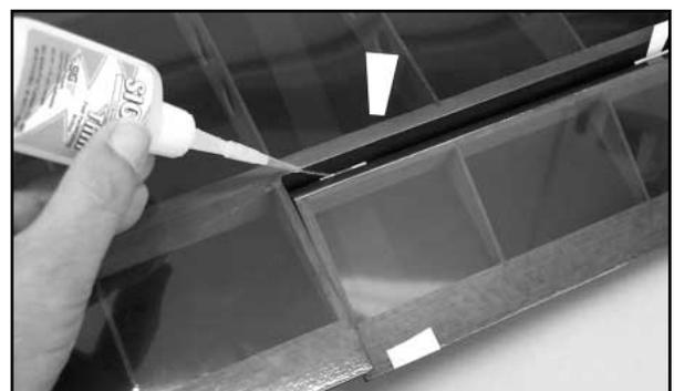
piece of masking tape. Remove the card wedge from one of the hinges and carefully apply four (4) drops of thin CA glue to each side of the exposed hinge - two (2) drops on each side of the die-cut slot. Note that using a fine applicator tip on the CA bottle is of great help in better controlling the flow of glue. Remove the card wedge from next hinge and once again apply four (4) small drops of CA glue to each side of the exposed hinge. Remove the last card wedge and apply CA glue to the hinge.
