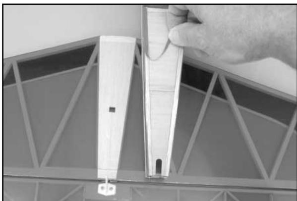
onto the stabilizer. Use a sharp #11 blade to lightly cut and then, remove the covering from the bottom center section of the stabilizer, trimming it approximately 1/16" inside of the marks just made. Likewise, trim away the excess covering material from the fuselage stabilizer platform, leaving about 1/16" or so of overlap.
