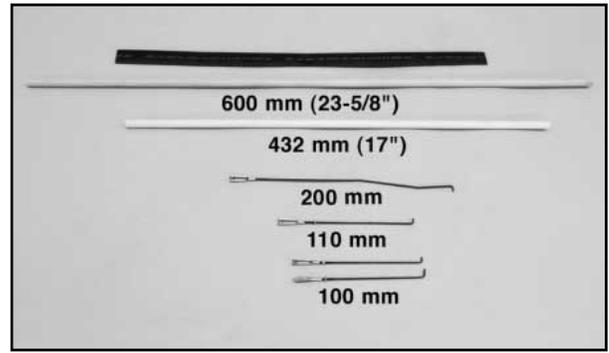
□ 1) The rudder pushrod assembly is made first. This pushrod will require the 17" wood dowel, the 200 mm threaded one end wire pushrod and one of the 100 mm wire pushrods with an RC link at one end. Note that the 17" wood pushrod is grooved and drilled at each end. These grooves are there to locate and nest the wire pushrods at each end. Also, note the 90° bends in the wire pushrods, made to fit into the pre-drilled holes in the wood pushrod.
