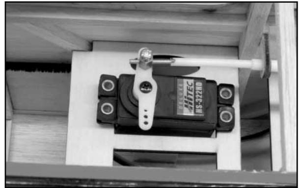
Adjusting the nose wheel to allow the model to roll perfectly straight along the ground can now be accomplished by simply adjusting the nose gear pushrod at the pushrod connector on the rudder servo output arm. Unplug the flight battery and turn off the transmitter.
