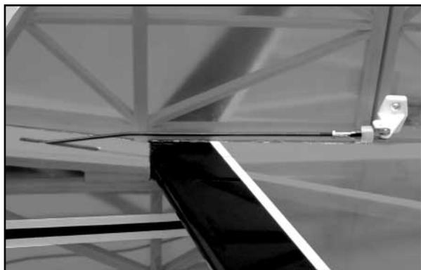
□ 6) With the pushrod now connected to both the rudder and the rudder servo, thread both lock nuts up to the rear barrel of the RC links and tighten them firmly. As shown, we installed short lengths - 1/4" or so - of fuel tubing over the RC links to hold them firmly in place.
