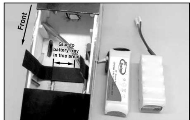
□ 8) As shown, the battery pack access hatch is held in place with a nylon landing gear strap mounted to the fuselage bottom with a T2.6 x 12 mm PWA screw. Locate these two parts from your kit contents.
