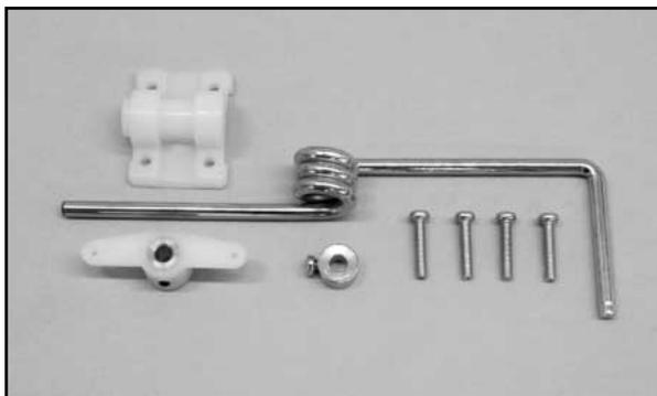
Note that this molded part has a spacer molded on one end. This spacer is the top of the bearing. When the bearing is correctly in place, this molded spacer is facing up toward the top of the fuselage, as shown. Install the nylon nose gear bearing to the bottom of the fuselage firewall, using the four provided M3 x 15 mm Phillips head bolts. Tighten these bolts firmly.
