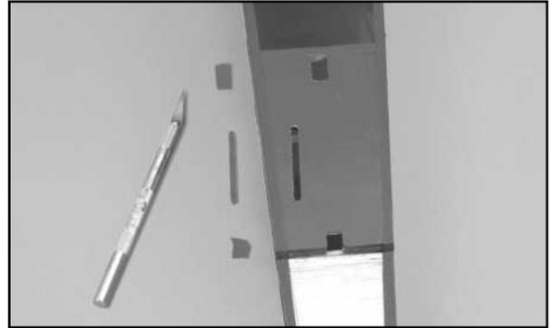
□ 2) The rudder is now hinged to the vertical fin and the elevators are hinged to the horizontal stabilizer. The method used for hinging these surfaces is exactly the same as the ailerons hinged earlier in this manual.
