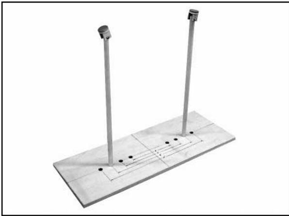
Properly balanced at the 3-1/4" point, the airplane should hang perfectly level. If the nose is down, the airplane is nose heavy. Likewise, if the tail hangs down from level, it is tail heavy. If either of these conditions exist, they must be corrected.
