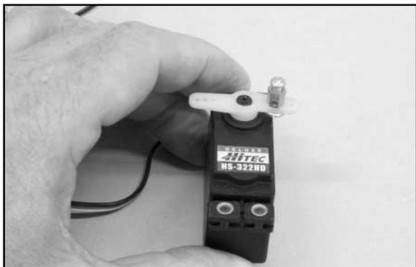
□ 5) The rudder pushrod assembly is now installed. To feed the rudder end of the pushrod through the pushrod exit slot at the top rear of the fuselage, it is first necessary to remove the RC link and lock nut from the longer rear pushrod wire. As shown, slightly bend the pushrod wire up to access the pushrod slot from inside the fuselage.
