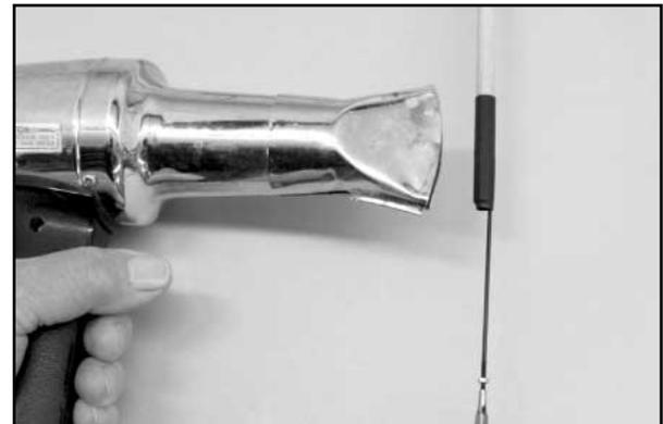
to shrink it firmly over the wire and wood joint. Use the second piece of heat shrink tubing to cover and secure the opposite end of the pushrod.
