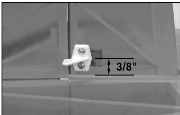
□ 4) The elevator control horn is attached to the bottom leading edge of the elevators at the exact centerline. The control horn is positioned on the bottom of the elevators with the arm facing forward and its connection holes aligned with the hinge line. Again mark and drill two mounting holes for the horn and harden the two holes with a drop of thin CA glue. Mount the horn in place with the provided T2 x 6 mm PWA screws.
