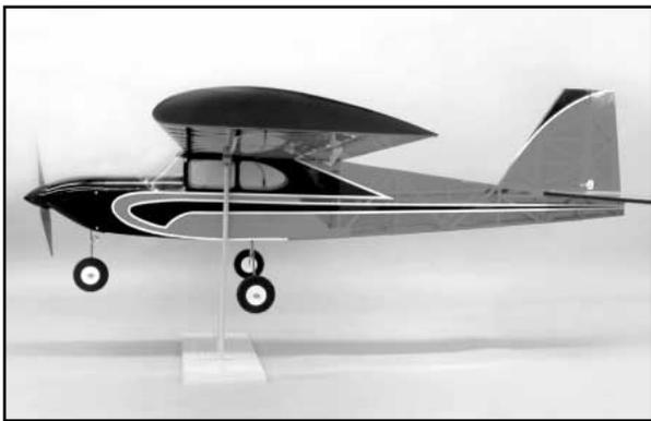
If the model is just slightly nose heavy; it can be safely flown. However, if it is very nose heavy, shift the flight battery pack battery to the rear until proper balance is achieved. Mark this battery pack location on the battery tray. This allows you to install the battery pack in the same location each time you fly the model.
