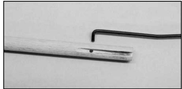
□ 2) Use 5-minute epoxy to glue the short 90° bent ends of each pushrod wire into the grooves and drilled holes on each end of the 17" wood pushrod.
