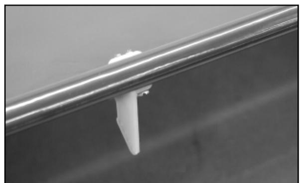
□ 6) Place the 4-40 Solder R/C Link into the last hole in the control horn. Swing the aileron pushrod against the control horn. Make sure that the servo is still in the neutral position and tape the aileron into approximately neutral position. Hold the pushrod against the 4-40 Solder R/C Link. Mark the pushrod wire 3/16" beyond the end of the center barrel of the solder link.
