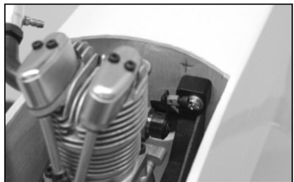
Now, remove the motor and drill a 1/8" hole in the firewall at the marked location. You will also need to drill a new hole in the fuselage frame that is at the front of the wing if the new location on the firewall is on the opposite side than the factory installation. The
