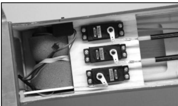
□ 8) Remove the cable and cut it at the mark just made (use a carbide cut-off wheel for this cut) and reinsert it back into the throttle housing tube in the face of the firewall. Solder the link in place to the trimmed end of the cable. Connect the solder link to the servo output arm and the nylon R/C link to the carburetor throttle arm. Use the radio to test the throttle action and adjust as needed to obtain true "low" and "high" throttle movement without any binding.
