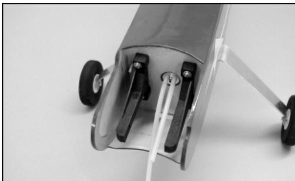
□ 4) Use a punch or pencil to mark the engine's mounting screw locations directly onto the motor mount arms. Remove the engine
