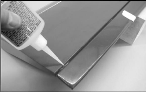
After sufficient time has passed, flex the aileron up and down several times to create free and easy movement. You must also pull on the aileron at each hinge location to be sure that the hinges are firmly bonded in place. Repeat this process to attach the aileron to the other wing.
