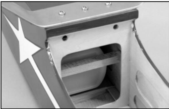
**NOTE:** The engine compartment was fuel proofed during production of the airplane. However, for a little extra insurance, you could give the engine compartment an additional coat of surfacing resin. If you decide to do this, use a brush to apply the resin and be sure to brush the resin up to the covering edges.
