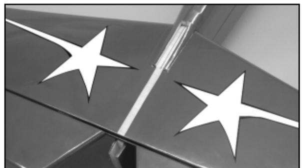
gluing. The covering should be trimmed away 1/16" inside the drawn lines. It is extremely important that you cut the covering only and not the balsa underneath. Do not cut into the balsa. Also remove the covering from the sides of the fin in the location of the tail fairings.
