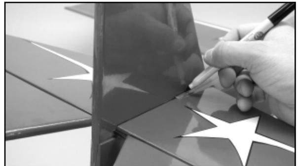
□ 11) You must now carefully remove the covering from the stabilizer and fin in order to expose the wooden structure for
