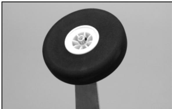
□ 2) The entire landing gear assembly is now mounted onto the bottom of the fuselage using the three M4 x 16mm Phillips Head Screws.
