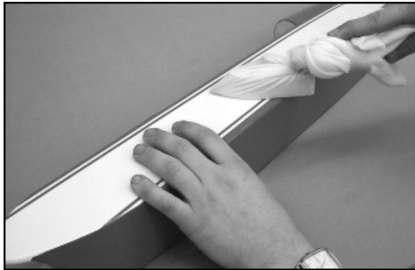
**MODELER'S TIP:** A very easy way to avoid damaging seams and joints when reshinking the covering is to protect the seams with wet paper towels rolled into strips. These are then arranged directly onto the joints or seams and their coolness protects the seam from shifting or "crawling" under heat.
