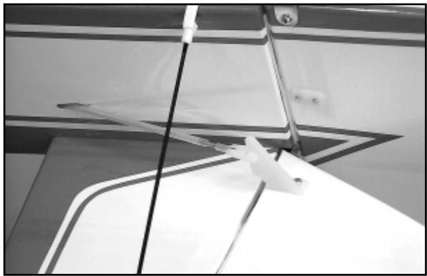
Install both the rudder and elevator pushrods into their exits from the rear of the fuselage and snap the R/C links in place to the nylon horns.
