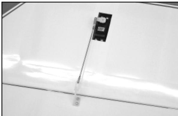
The nylon R/C link on the aileron pushrod can now be attached to the aileron horn. We typically use the second hole from the horn's tip for initial placement. With the servo and aileron now connected, the nylon R/C link can be adjusted to position the aileron in approximately "neutral". Final adjustments will come later.
