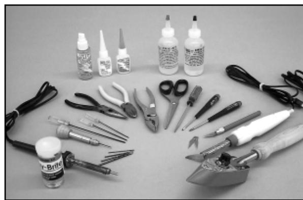
In addition you will also be required to make a few solder connections. We suggest that you have a good soldering iron and good quality solder and flux. For the pushrod connections, we use and like the Stay-Brite® Silver Solder product.
