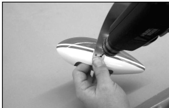
Remove the 7/64" bit from your power drill and replace it with a 9/64" dia. bit. Re-drill the two holes in each wheel pant with the 9/64" bit.
