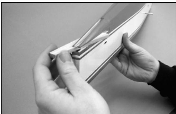
Use your hobby knife to cut the covering material away from the rear fuselage tailpost, exposing the rear fin slot.
