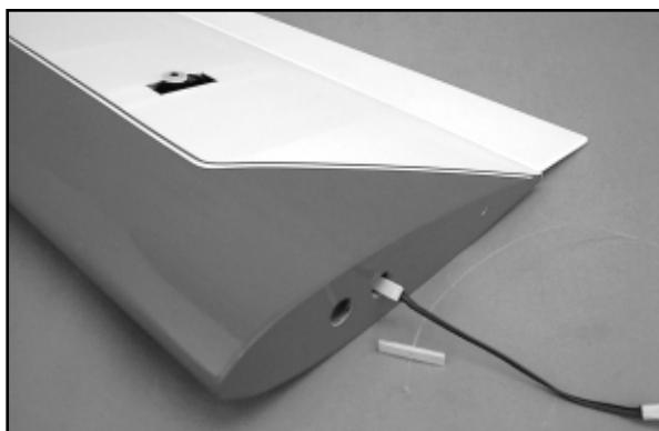
line and the servo cable lead through the wing until the servo cable emerges from the root rib.
