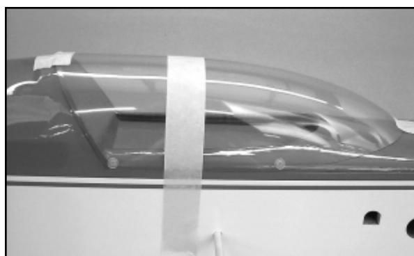
holes in the canopy (from experience, do not drop these washers on the floor because they are really hard to find!). Place the canopy onto the canopy hatch with its rear edge lined up with the rear edge of the angled former. Carefully center the canopy and use a few pieces of masking tape to hold it in this position. Use a pin through each washer's center to poke a small hole at each location. Remove the tape and the canopy.
