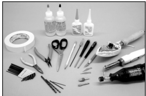
A selection of glues - thin, medium, and thick SIG CA, and SIG Epoxy Glue (5-minute and 30-minute)
