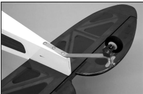
□ 5) Attach the aluminum spring centering horn to the bottom leading edge of the rudder, as shown, using two #2 x 3/8" screws. Note that the bottom leading edge of the rudder has hardwood beneath the covering as a hardpoint for the screws. Position the front edge of the horn 1/8" behind the leading edge of the rudder. Use the aluminum centering horn to first mark the required
