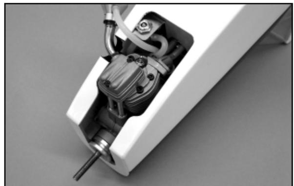
to the wood rail mounts - be sure to maintain the 1/16" - 3/32" spinner backplate clearance. Use medium fuel tubing (not supplied) to make the required connections between the engine and fuel tank and the vent line and the muffler manifold pressure nipple.
