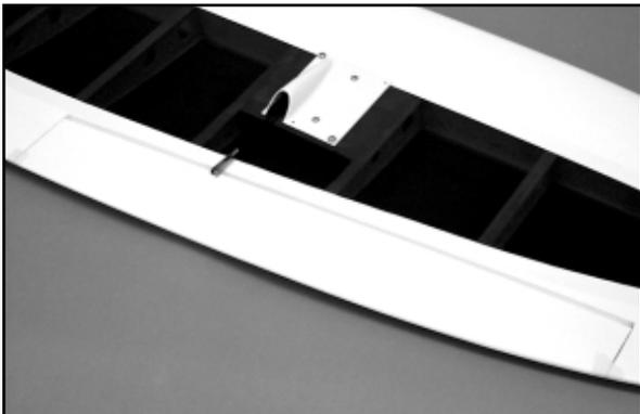
molded fairing in the servo tray, at 90° to the servo. Take off and reposition the output arm as needed to achieve this. With these two issues addressed, install and tighten the servo output arm screws in both servos. Carefully re-install the servo and tray back into the aileron servo bay opening in the wing panel and secure it in place with four #2 x 5/16" Phillips/Washer Head screws. Use a couple of pieces of masking tape to hold the aileron in neutral.
