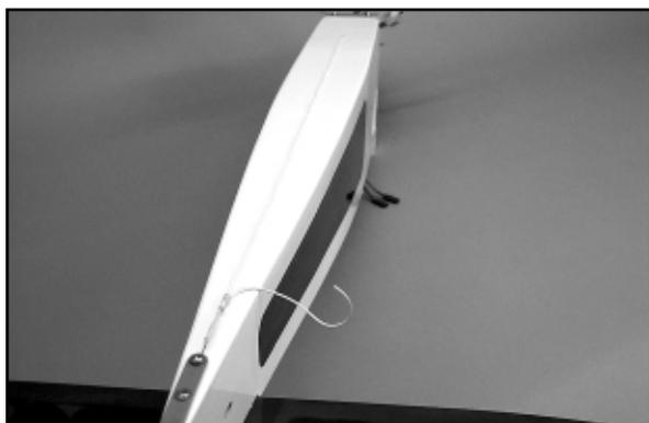
tailwheel bracket. We made a simple wire hook from a straight pin and attached it to the forward screw holding the bracket in place. We then used a rubber band to anchor the antenna along the bottom length of the fuselage.
