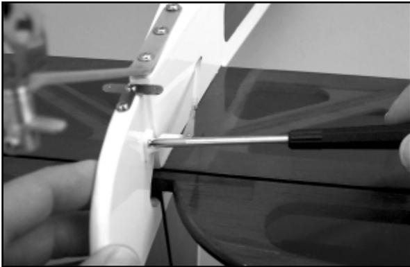
□ 2) Remove the pushrod tube from the fuselage. Re-insert the unprepared end of the pushrod into the fuselage from the servo compartment, with the stud and metal link at the rudder servo. Connect the metal link to the outer-most servo arm hole. Make sure the rudder servo is in "neutral" - turn the radio system on if necessary.
