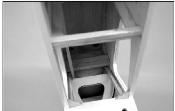
□ 11) Apply a little thread-locking compound to the threads of the 3.5 x 20mm mounting bolts. Install the lock washers onto each bolt, followed by the larger flat washers. Install the engine and aluminum rails into the engine compartment. Slip the four bolts (with washers) into the oblong holes in the aluminum rails. Thread the bolts into their blind mounting nuts and tighten the bolts firmly
