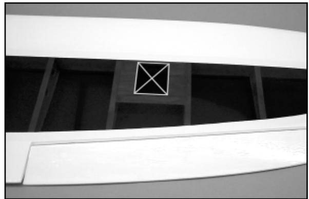
Use a covering iron to seal the four loose edges of each side of the servo bay opening and trim the excess covering material with a hobby knife. Inside the servo bay opening you will find a short length of wood with a string tied to it. This string is used to pull the aileron servo lead through the wing and out of the opening in the bottom of each wing panel - leave it in place for now.
