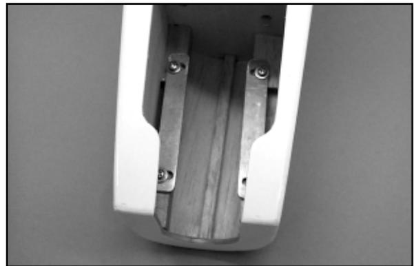
□ 2) Remove the muffler header pipe and needle valve from the engine. Fit the engine in place onto the aluminum rails. Slide the engine to its approximate mounting position with the prop hub just ahead of the front of the fuselage by approximately 1/16" - 3/32". This spacing will be the clearance for the spinner backplate
