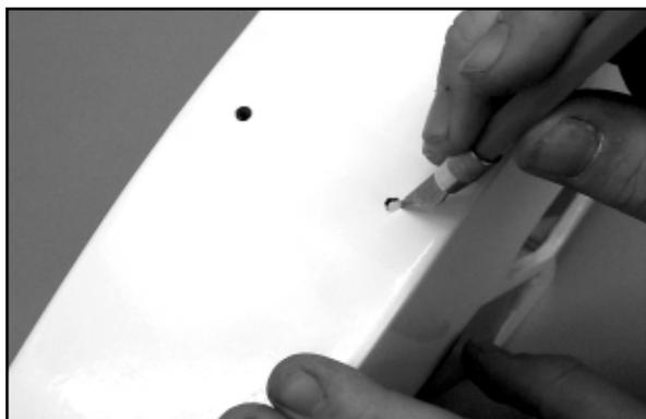
Last, you will need to remove the covering over the rudder and elevator pushrod exits. These are located on each side of the fuselage, beneath the horizontal stabilizer. A sharp #11 blade is perfect for this step. If necessary, use a covering iron to re-seal the covering around these openings.
