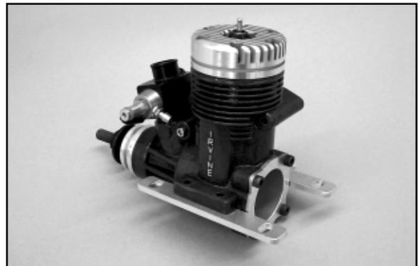
□ 5) Use a shortened pencil with a sharp point to mark the locations of the engines mounting holes onto the aluminum motor mounts. To remember which rail fits on the right and left side of the engine, mark them with an "R" and "L" (left and right).
