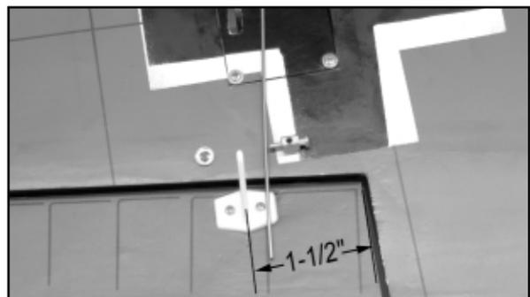
to its bottom surface. Repeat this process on the opposite aileron. Use the four M2 x 20 mm bolts and the two plastic control horn backing plate to now mount each aileron horn to the bottom of each aileron with the backing plates on top of each aileron to engage the bolt ends. Cut off the excess bolt ends and file smooth.
