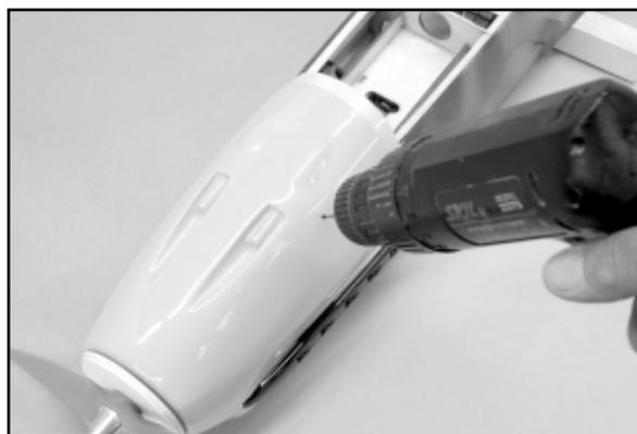
❑ 4) With a screwdriver, install the four cowl mounting screws through the holes in the cowl and into the plywood pads. Tighten the screws just enough to place the washer head in contact with the cowl - no more. Remove the pieces of tape, the propeller nut, the propeller, and the plywood backplate. Remove the 1/16" spacers from the rear of the backplate and lightly sand the backplate smooth.
