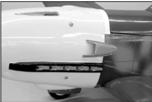
If desired, typical plastic paints can be used to add a little more detail and realism to the cowl. The two machine gun troughs on top of the cowl can be painted flat gray to simulate gunpowder staining. The molded gun barrels can be painted flat black. The two exhaust manifolds can be painted a smoky gray to simulate burning exhaust.
