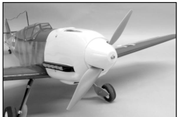
**Modeler's Note:** A standard 2-3/4" dia. yellow nylon spinner, such as a SIG # SIGSP2755, can be used to make a nice looking alternative spinner, by simply cutting off 1/2" from the tip of the spinner cone.
