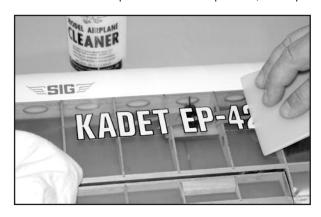
stiff cardboard (or sheet balsa, thin plywood, or a SIG SH678 EPOXY SPREADER) to squeegee the excess liquid out from under the decal. Squeegee repeatedly, removing all excess liquid and any air bubbles. Mop up the liquid with a paper towel. Allow to dry overnight.
