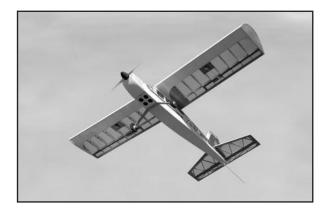
The KADET EP-42B has very mild stall characteristics - straight ahead with a slight nose drop, resuming flight almost immediately. It can also be banked fairly sharply with little tendency to "fall off".
