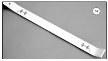
6) Mount the Front and Rear Float Struts along with the Spreader Bars to the plywood mounting flanges of the floats, using the M4 x 20 mm Socket-Head Bolts, M4 Flat Metal Washers, and M4 Lock Nuts provided. Put the flat washers under the head of the bolts. The lock nuts don't need washers since they bear on the aluminum struts. Snug the bolts and nuts, but do not tighten them completely until later.
