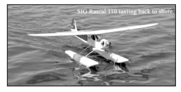
You will also find that many float planes will turn much better to the left than they do to the right due to engine torque. Sometimes, if you're having trouble turning the model to the right to point it in the direction you want to go, try making a wide left turn all the way around the other way.
