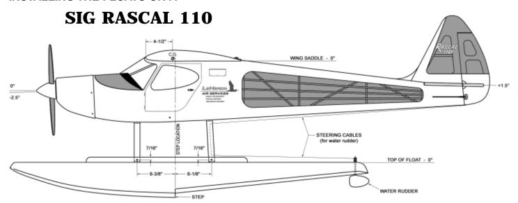
1) The standard Balance Point (or C.G.) for the Rascal 110, as specified in its assembly manual, is 4-1/2" behind the leading edge of the wing. This is the balance point recommended for flying this airplane from land, and it is the same balance point we recommend for float flying. If your Rascal 110's balance point is not currently at 4-1/2", we recommend that you rebalance your airplane at that C.G. location at this time.
